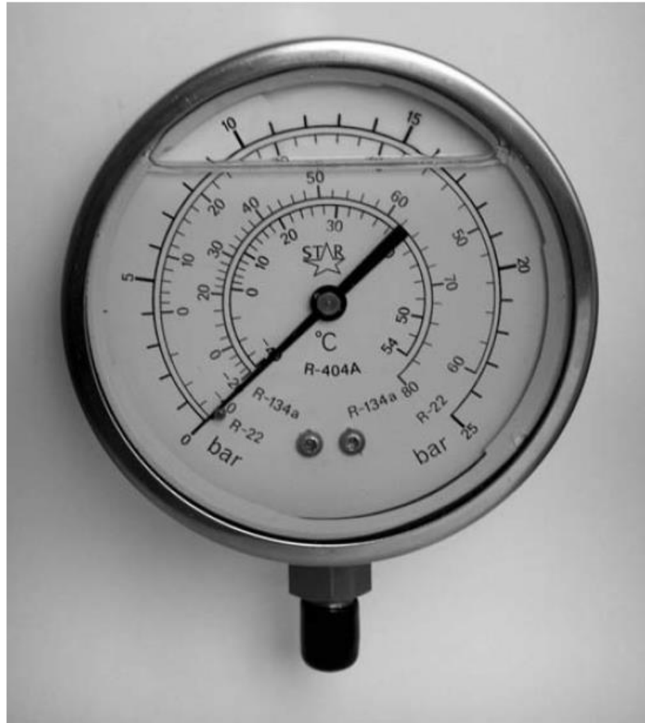
Figure 9.5 Refrigeration pressure gauge (Star Instruments)
